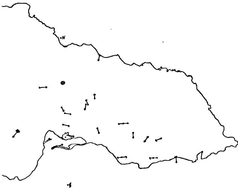
FIG. 8.—ARROWS SHOWING FALL OF BUILDINGS.
